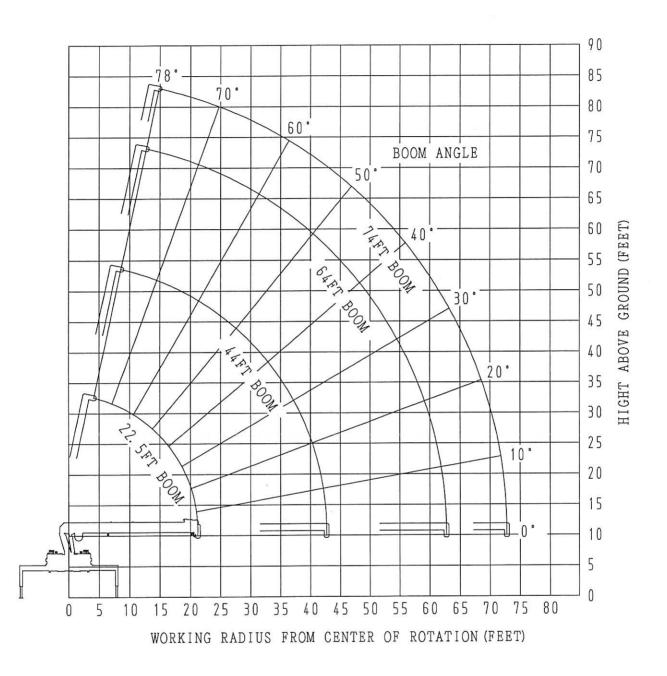
Note : The above figures are based on no-load condition and do not include the deflection of the. boom.
